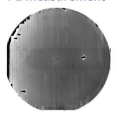
Only one triangle defect can be detected by visual
